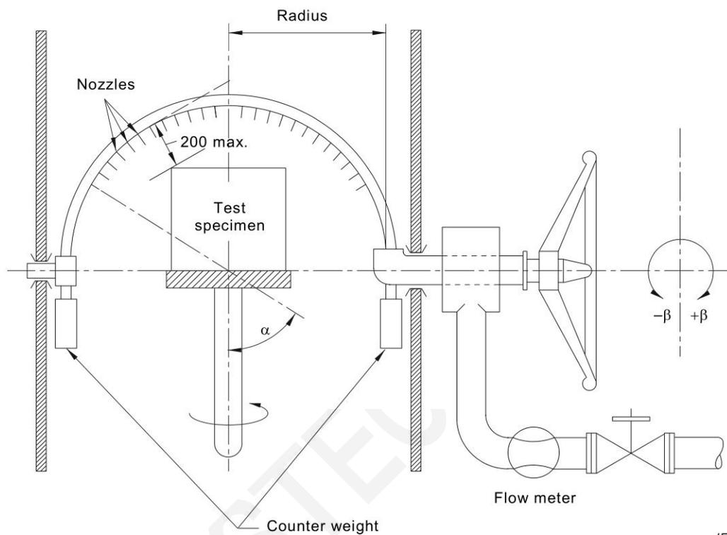
NOTE 1 The nozzles have a centre-to-centre distance of 50 mm.
